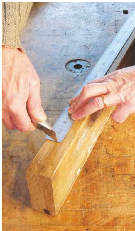
▲ Pic.11 Marking the haunch shoulder
